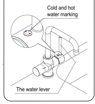
2. Hold the lever and turn up or down as directed by the arrow to choose hot or ambient water.
