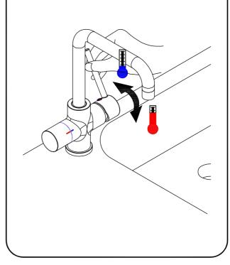
3. Pull the lever to the right as shown by the arrow for the water to flow out.
